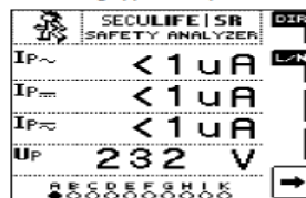
Display of current of applied parts – Display of measurement type/ mains polarity – Selecting application part
